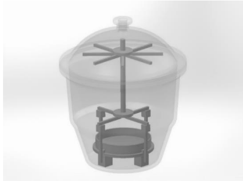
Figure 4. Representation of a Flowers of Sulfur Test Chamber
