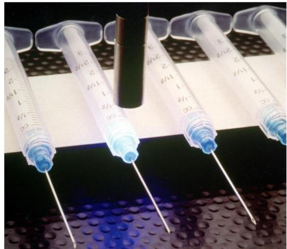
Figure 5. Adhesive Undergoing Cure
