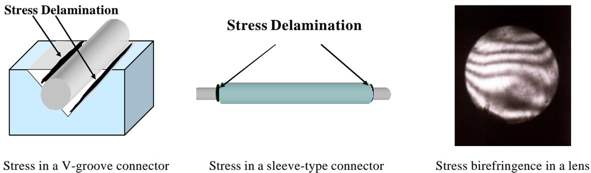
**Figure 1.** Adhesive induced stress, either from shrinkage on cure, aging, or thermal excursions can cause birefringence or delamination failures. Overly rigid materials may not relieve the stress from divergent coefficients of thermal expansion (CTE) which can manifest themselves in substrate delamination or in substrate distortion.
