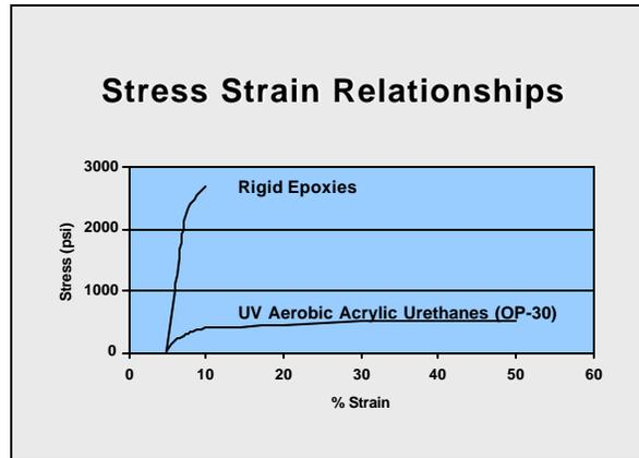
Shrinkage and modulus are major components of stress on cure. Table 2 illustrates how induced stress may exceed the strengths of the substrates. The result can be delamination or movement between bonded parts. Equation 1 below is a first approximation to estimate stress on cure. Table 2 illustrates calculations.
