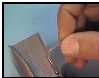
Figure 8. Removal of a Peelable Masking Resin
