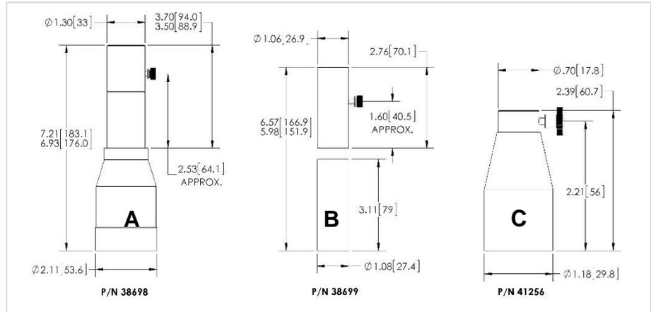
Figure 9. Rod Lens Dimensions
