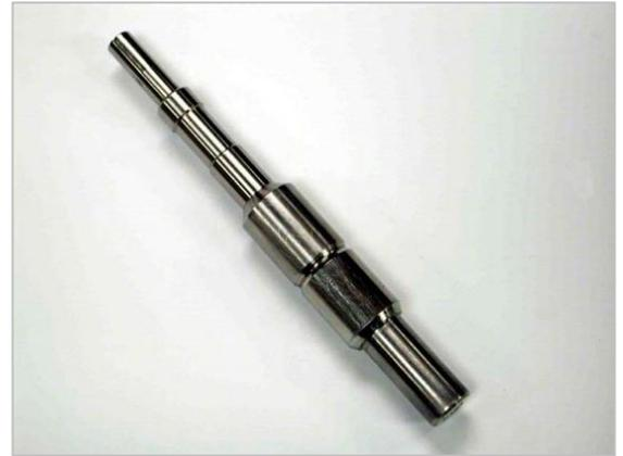
Figure 4. Lightguide Simulator
