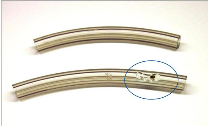
The image above compares parts exposed to conventional (bottom) and LED (top) light-curing energy sources. Exposure parameters:
