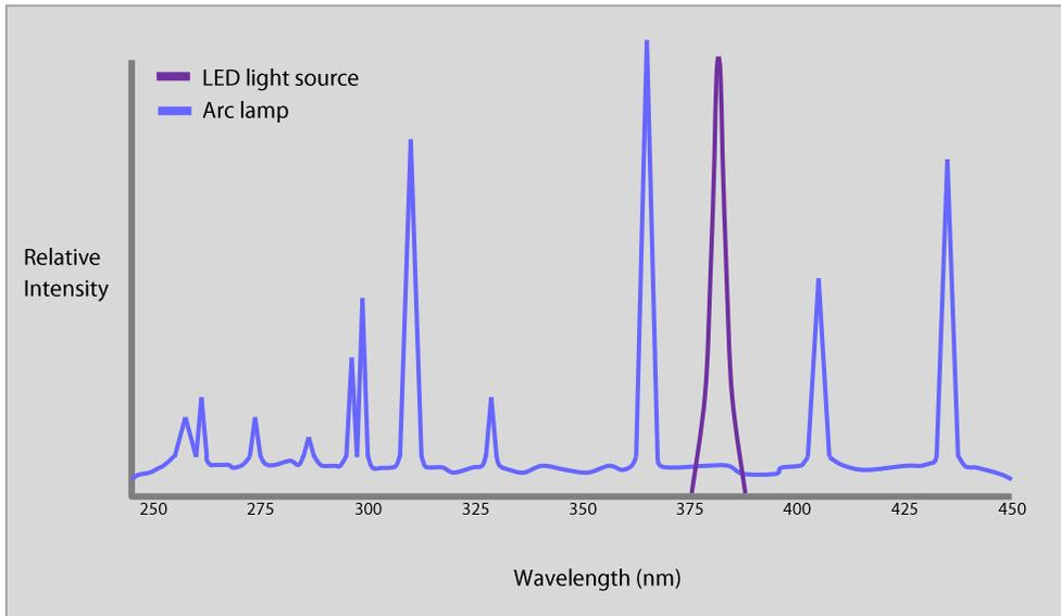
It is essential to match the wavelength of the LED-curing lamp with the adhesive photoinitiator's absorption spectrum. This pairing is dependent on having an optimized solution.
