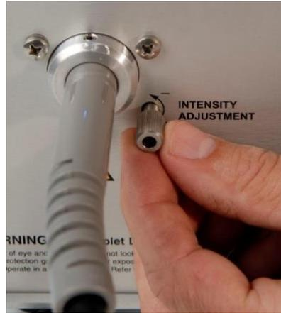
**3) Maintain a Consistent Distance from the Lightguide to the Part** – Intensity varies dramatically with distance from the end of a lightguide.
