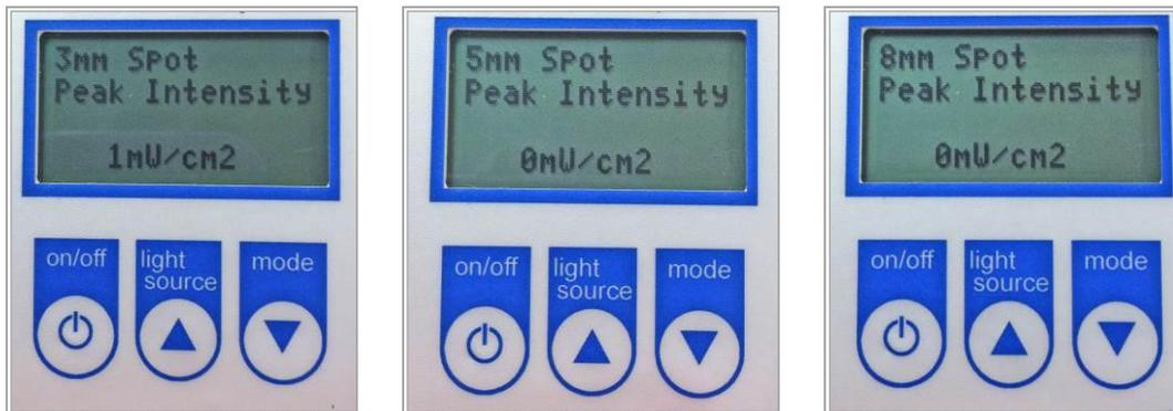
7. Press and release the Mode button to select the operating mode. The different operating modes are:
