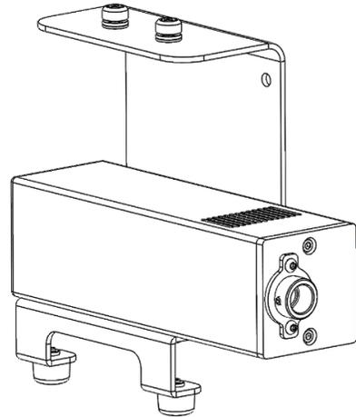
2. Attach the mount to the controller - Using the supplied hex wrench, tighten the 2 screws through the mount and into the controller mounting holes.
