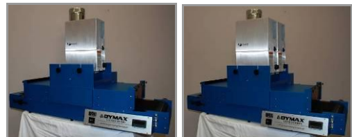
Figure 5. Conveyor with Lamp(s) Installed
