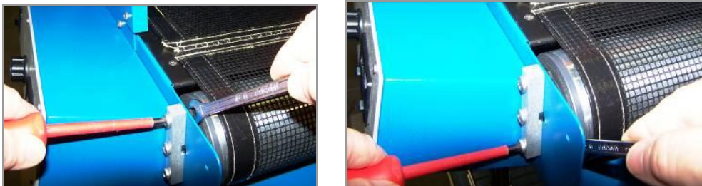
Figure 25. Loosening Drive-Roller Shaft-Support Fasteners
