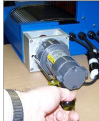
Figure 46. Reinstall Pinch Guard
