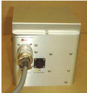
Figure 14. Attach the Lamp Connector Cord
