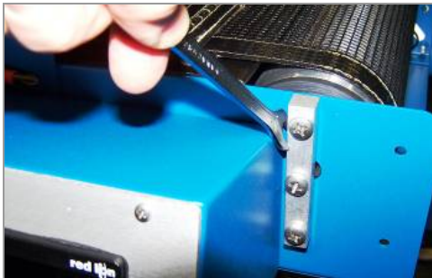
Figure 43. Move Shaft Assembly to Center Belt
