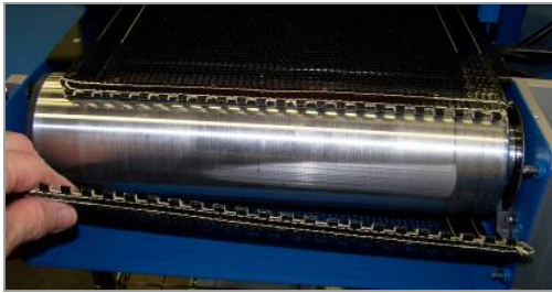
Figure 37. Run New Belt Around Conveyor Frame
