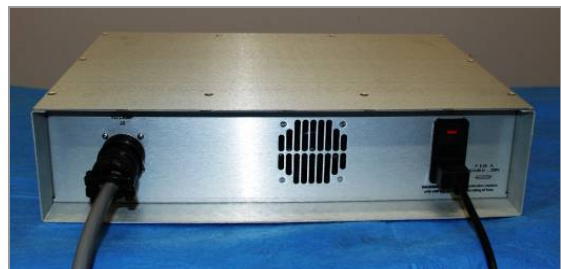
Figure 17. Attach Lamp Connector Cable to Power Supply
