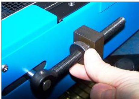
Figure 39. Tighten Belt Tension Knob
