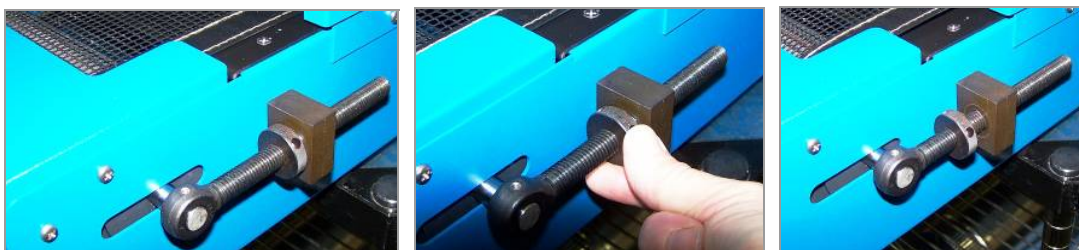
Figure 32-34. Back Off the Belt Adjustment Knob
