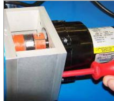
Figure 30. Remove M4x25 Screw
