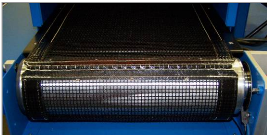
Figure 18. Position Belt Slice at End of Conveyor
