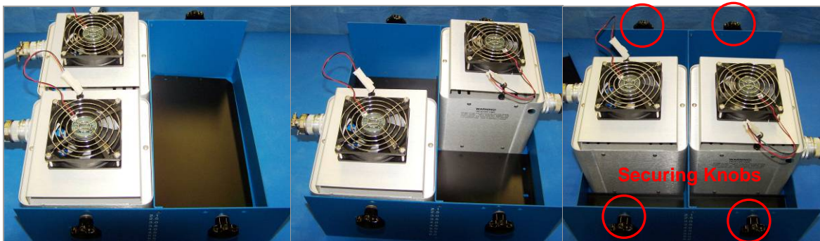
Figure 5. Upper Lamp Support Housing with Two Lamps – Three Possible Configurations
