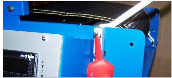
Figure 24. Tighten the Drive Roller Shaft Support Support Fasteners (bottom)
