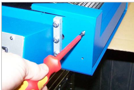
Figure 25. Reinstall the Pinch Guards (left)
