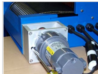
Figure 26. Reinstall the Pinch Guards (right)
