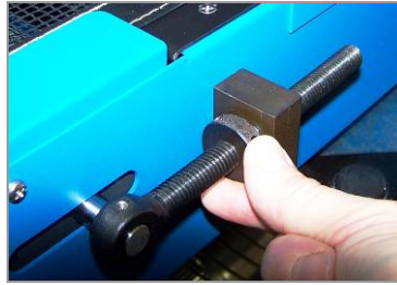
Figure 15-17. Back off Belt Adjustment Knob
