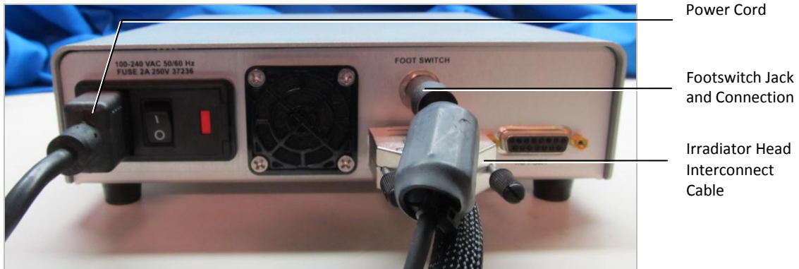
Figure 7. Installing Cables on the Back Panel of the Controller
