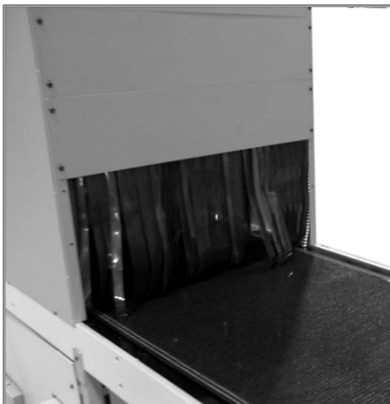
Figure 9. Conveyor Curing Chamber Entrance
