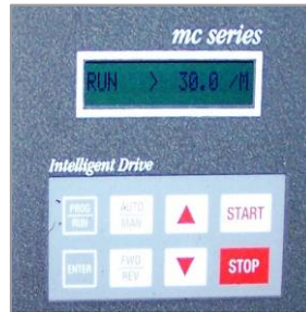
Figure 12. Conveyor Speed Controller
