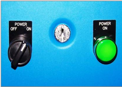
Figure 11. Main Power Controls
