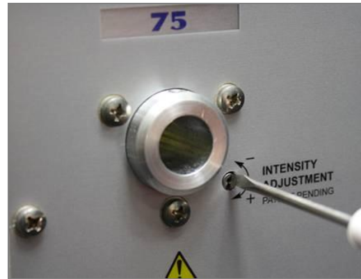
Figure 7. Adjusting Intensity with Screwdriver
