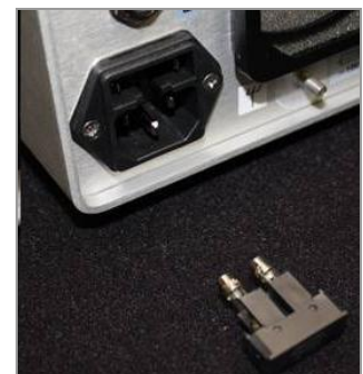
Figure 19. 4.0 Amp Fast-Acting Fuse (PN 37869)
