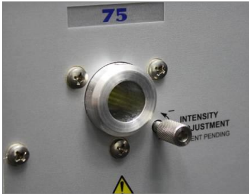
Figure 6. Intensity Adjustment Knob Screwdriver
