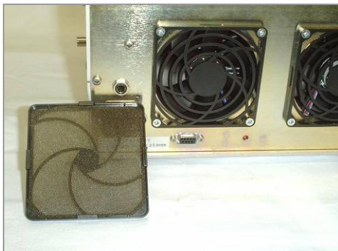
Figure 28. Exhaust Fans with Fan Filters Removed
