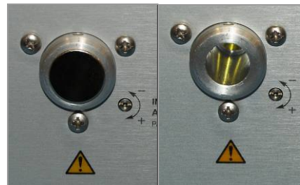
Figure 4. Lightguide Mount Protective Cover Installed (left); Protective Cover Removed (right)
