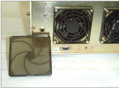
Figure 28. Exhaust Fans with Fan Filters Removed
