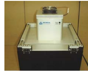
Figure 9. 5000-EC Reflector Housing Mounted on Light Shield
