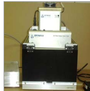
Figure 13. 5000-EC Reflector Housing Mounted on ZIP™ Shutter and Light Shield
