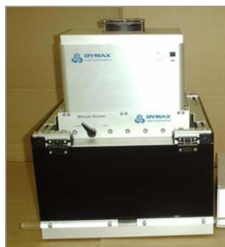
Figure 14. 2000-EC Reflector Housing Mounted on Manual Shutter and Light Shield
