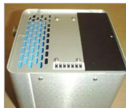
Figure 16. Temperature Control Plate and Temperature Indicating Strip, installed
