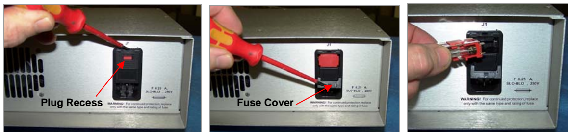
Figure 12-14. Replacing Fuses in the Power Supply
