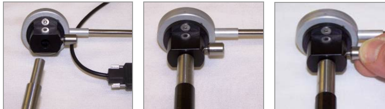
Figure 7-9. Attach Lightguide Adapter to Lightguide (Step 4)
