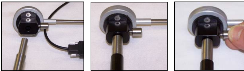
Figure 7-9. Attach Lightguide Adapter to Lightguide (Step 4)
