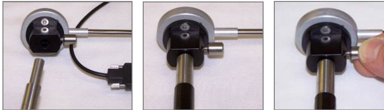
Figure 7-9. Attach Lightguide Adapter to Lightguide (Step 4)
