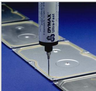
Appliance Casing FIP/CIP Gasket
