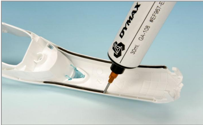
Dispensing gasket bead onto appliance handle
