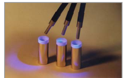
Trifurcated wand curing metal-to-plastic assembly
