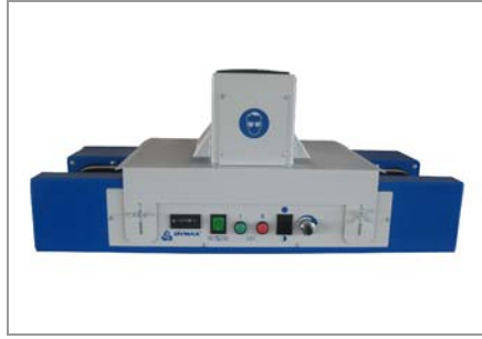
DYMAX UVC-5 Conveyor System is equipped with a 120 mm wide belt. Curing time can be adjusted by changing the belt speed from 1.4 to 11 meters per minute continuously. CE Marked.
