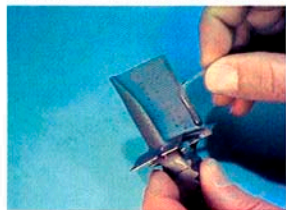
Removal of a Peelable Masking Resin
